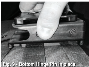
Fig. 9 - Bottom Hinge Pin in place
